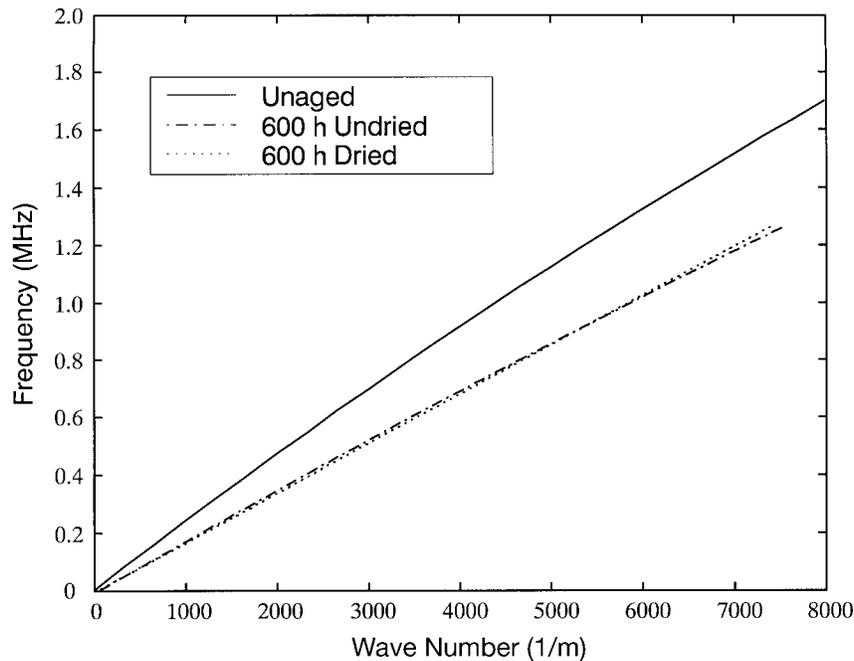
FIG. 7. Comparison of Rayleigh Dispersion Curves for Unaged, 600-h Undried, and 600-h Dried (Aging at 84°C)
