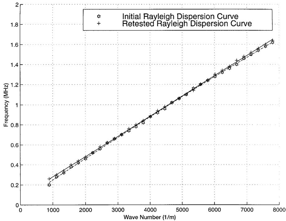
FIG. 5. Comparison of Rayleigh Dispersion Curves for Same Control Volume That Demonstrates Repeatability of Measurement Procedure
