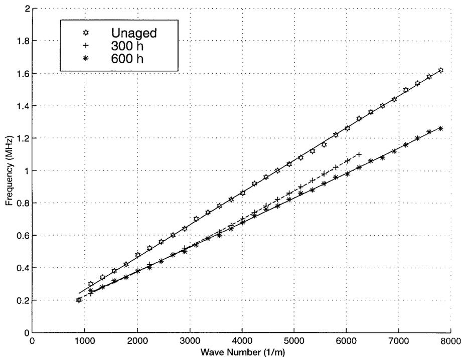
FIG. 6. Comparison of Rayleigh Dispersion Curves for Unaged, 300 h, and 600 h at 84°C Temperature
