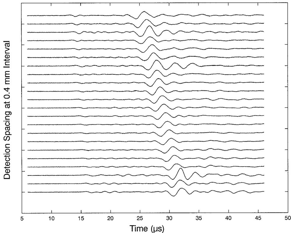
FIG. 3. Comparison of 22 Typical Waveforms with Propagation Distances Varying from 27.4 to 36.2 mm (with  $\Delta x = 0.4$  mm)
