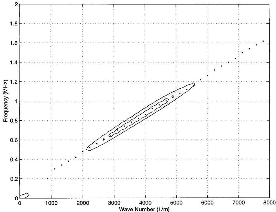
FIG. 4. Contour Plot of Frequency versus Wave-Number Spectrum plus Local Maxima
