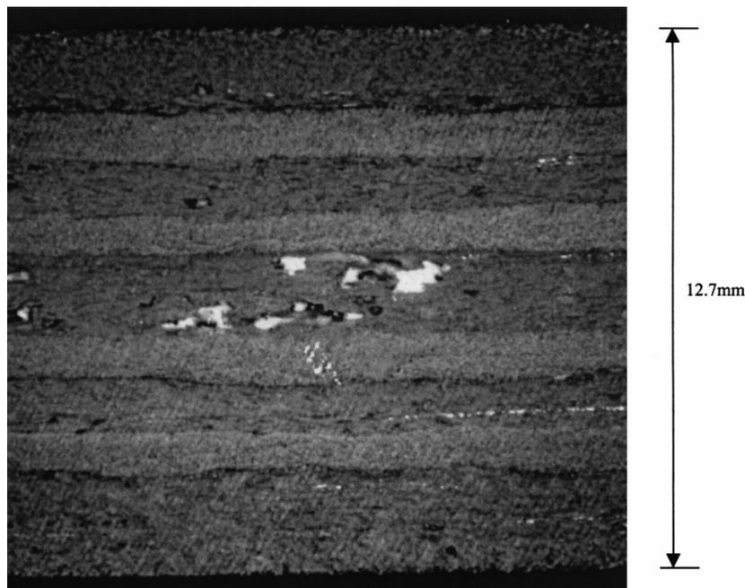
FIG. 1. Magnified Digital Image of Typical FRP Cross Section
